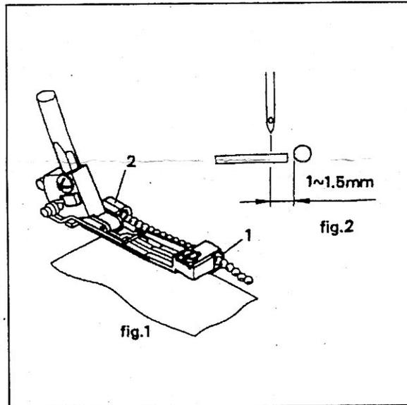
The Beading Foot is used for sewing on beads, sequins, pearls and thick cord.
